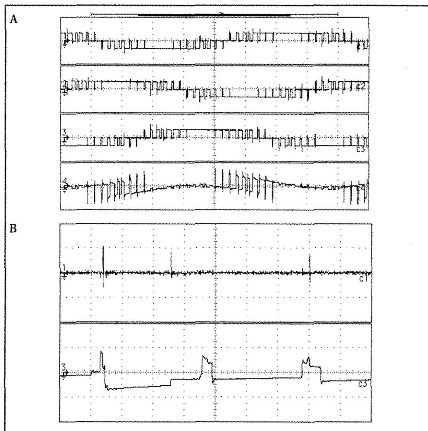
Figure 1. 5 hp, 460 V (A) (Ch. 1-3) PWM motor input voltages (L-L, 500 V/div), (Ch. 4) shaft voltage (10 V/div) (B) Outboard bearing current (50 mA/div), and shaft voltage (10 V/div).
