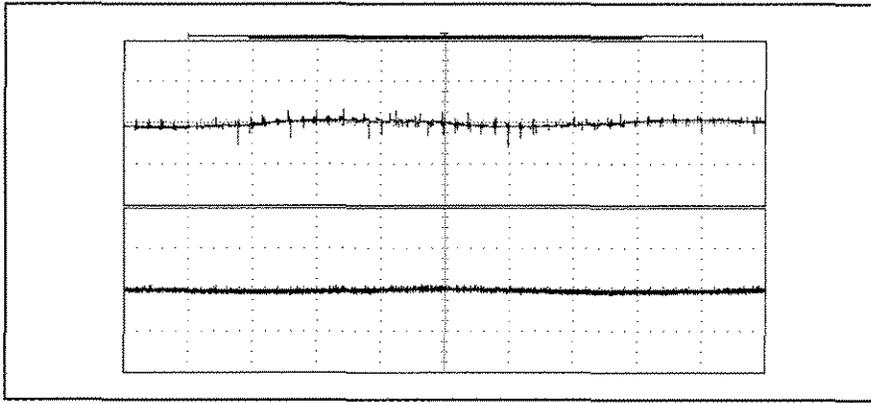
Figure 4. Shaft voltage (top, 4 V/div) and bearing current (bottom, 200 mA/div) with dual-bridge inverter driven motor.
