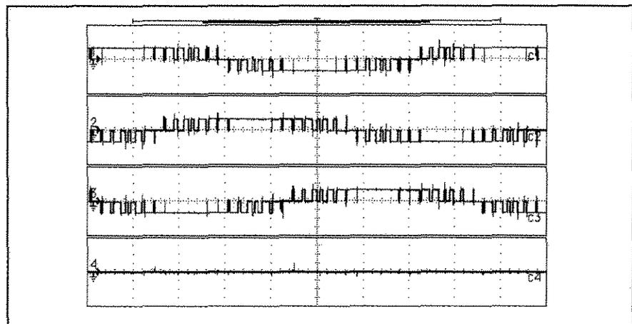
Figure 2. 5 hp, 460 V, (Ch. 1-3) PWM motor input voltages (L-L, 500 V/div), (Ch. 4) shaft voltage (negligible) with shaft grounding system (4 V/div).
