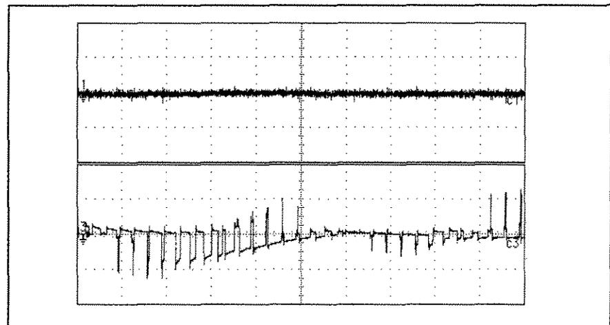
Figure 3. 5 hp, 460 V, Outboard bearing current (negligible) with ceramic bearings or insulated bearings (200 mA/div), and shaft voltage (4 V/div).
