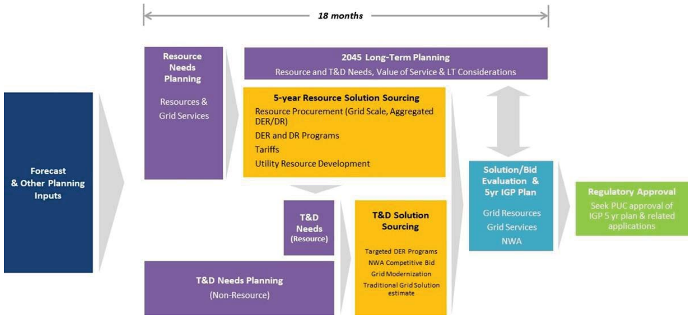
Figure 3: Integrated Grid Planning & Solution Sourcing Process
